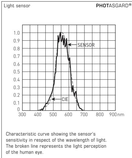
The sensor used in **PHOTASGARD®** light intensity sensors was specifically adapted to the sensitivity of the human eye. Its greatest sensitivity is in the range of 350 nm to 820 nm. Therefore with its special filter the sensor is predestined for exposure measurement of daylight and/or for measuring artificial light of high colour temperature (similar to sunlight).
