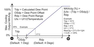
Pipe temperature (calculated by Dew Point Offset - OSdp and Dew Point Range - Rdp parameters).
