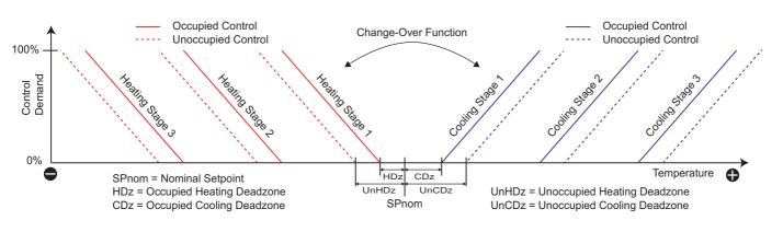
The multi-stage temperature control loop can be configured to control built-in temperature, Universal Input 1 temperature/voltage, Universal Input 2 Temperature/voltage, or network value (network temperature).
