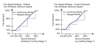
Fan Speed Settings : Default. Except Fan Off Mode Fan Off Mode: Off (Fan Off at 0% Demand)
