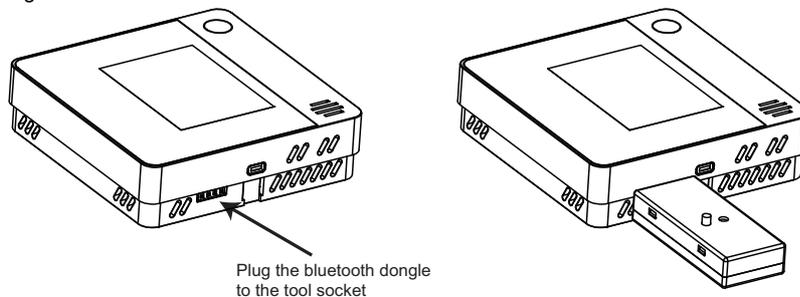
To connect the TDR/QDR20 to Zone 2 change the device address to 2 using using the abovementioned tools, or through the display menu.
