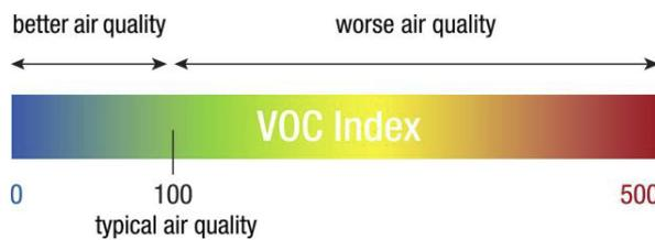
Measured air pollutants include harmful gases (acetone from paints and glues, toluene from furniture, mattresses and building products), other gases (ethanol from alcohol, perfumes and cleaners), odours (hydrogen sulfide and volatile sulfuric compounds from rotten food and farts; ammonia and amines from pet urine), smoke (benzene and nitrosamines from cigarette smoke).
