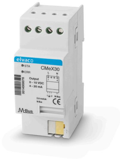
The CMeX30 is a digital to analog converter with an output voltage range from 0 to 10 V or current output range from 0 to 20 mA. It features standard M-Bus over IR communication and is equipped with the unique IR-Pass Through function, making the product series stackable.
