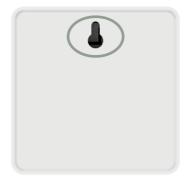
**Caution:** When using a screw for mounting, please make sure that the total length protruding from the wall does NOT exceed 6 mm. Not adhering to this advice might result in physical contact between the screw and internal parts of the sensor causing a loss in range or malfunctioning of the sensor.
